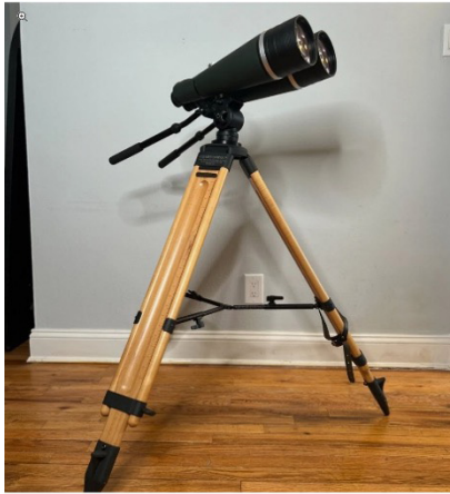
25x100mm Binoculars on a TR3 Maple legged tripod from eBay. The black pipes are spreaders that keep the tripod legs from splaying apart.
