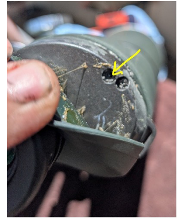
Peeling back the rubber cement holding the rubber cover reveals the collimation hole, one on each side.
