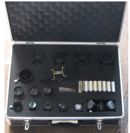
Eyepiece Case #5: Black case, Eyepieces: : 2" Celestron E-Lux 40mm, Meade 2" QX 26mm, 1.25" VLW 13mm, VLW 17mm, Orion 9mm Plossl, Orion 6mm Kellner, Unknown 32mm, Unknown 25mm, Ortho, 20mm Kellner 20mm, Unknown crosshair, 1.25", Kellner .965", Other: 2" Extension Tube, 1.25" extension tube, 2" Nebula filter,
