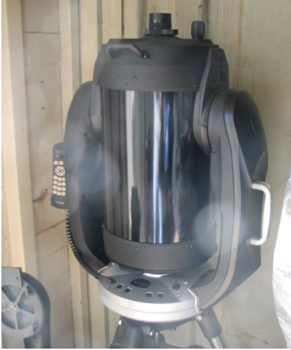
Celestron 11" CPC series Alt-Az fork mounted, with tripod and GOTO. We have 2 of these telescopes.
