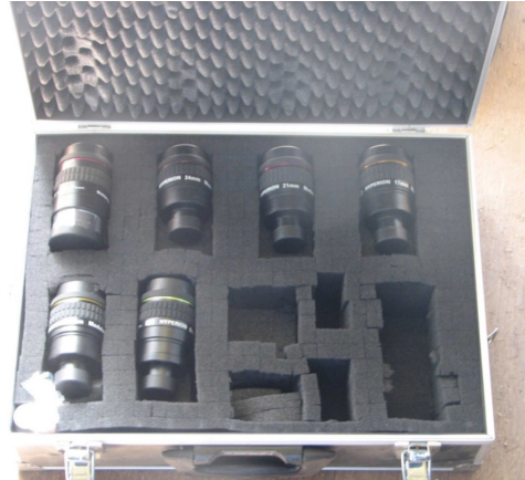
Eye piece case No. 2 Black Orion Case contains a 2" Hyperion-Aspheric 72-degree 36mm and 1.25" Hyperion eyepieces: 8mm, 13mm, 17mm, 21mm, and 24mm.
