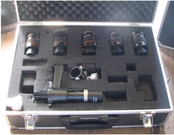
Eye Piece Case #1: Black Orion Case 5 1.25-inch Celestron Multi Coated X-Cell LX eyepieces: 25mm, 18mm, 12mm, 9mm, 7mm focal lengths. 6x30 finder and diagonal.
