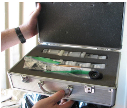
Eyepiece Case #6. Small Silver case 8 Meade Super Plossl 1.25" eyepieces. Focal Length: 40mm, 32mm, 26mm, 20mm, 15mm, 12mm, 9.7mm, 6.4mm, 12mm Illuminated reticle, 1.25" eyepiece 1.25" diagnol.
