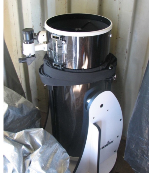
Orion SkyWatcher 12" Collapsible Dobsonian with 8x50 finder
