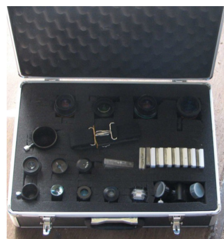
Eyepiece Case #5: Black case, Eyepieces: 2" Ce- lestron E-Lux 40mm, Meade 2" QX 26mm, 1.25" VLW 13mm, VLW 17mm, Orion 9mm Plossl, Orion 6mm Kellner, Unknown 32mm, Unknown 25mm, Ortho, 20mm Kellner 20mm, Unknown crosshair, 1.25", Kellner .965", Other: 2" Extension Tube, 1.25" extension tube, 2" Nebula filter,
