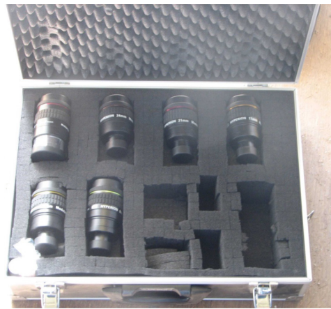
Eyepiece case No. 2 Black Orion Case contains a 2" Hyperion-Aspheric 72-degree 36mm and 1.25" Hyperion eyepieces: 8mm, 13mm, 17mm, 21mm, and 24mm.
