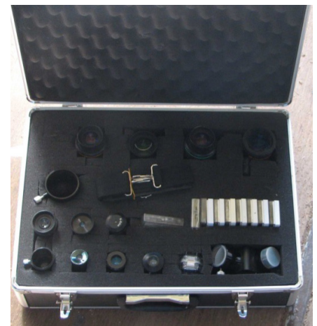
Eyepiece Case #5: Black case, Eyepieces: : 2" Celestron E-Lux 40mm, Meade 2" QX 26mm, 1.25" VLW 13mm, VLW 17mm, Orion 9mm Plossl, Orion 6mm Kellner, Unknown 32mm, Unknown 25mm, Ortho, 20mm Kellner 20mm, Unknown crosshair, 1.25", Kellner .965", Other: 2" Extension Tube, 1.25" extension tube, 2" Nebula filter, 3x Barlow, 1.25" Orion diagonal dielectric mirror.
