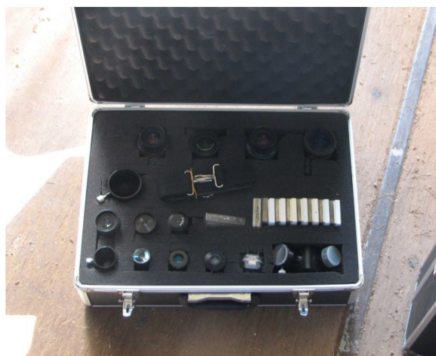
Eyepiece Case #5: Black case Eyepieces: : 2" Celestron E-Lux 40mm, Meade 2" QX 26mm, 1.25" VLW 13mm, VLW 17mm, Orion 9mm Plossl, Orion 6mm Kellner, Unknown 32mm, Unknown 25mm, Ortho, 20mm Kellner 20mm, Unknown crosshair, 1.25", Kellner .965", Other: 2" Extension Tube, 1.25" extension tube, 2" Nebula filter, 3x Barlow, 1.25" Orion diagonal dielectric mirror
