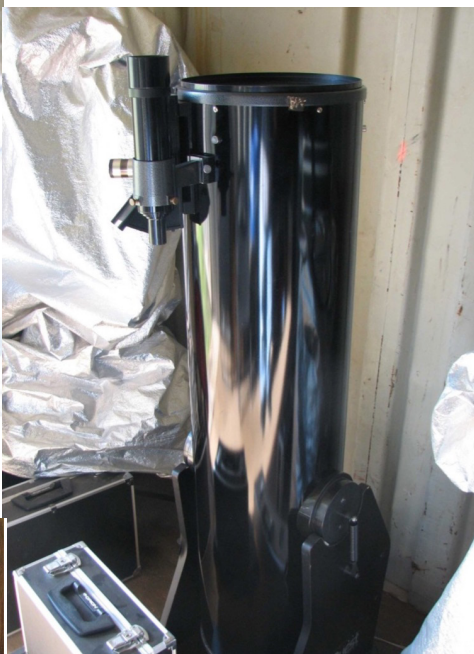
Orion SkyQuest 10" Dobsonian with Telrad and 8x50 finder.
