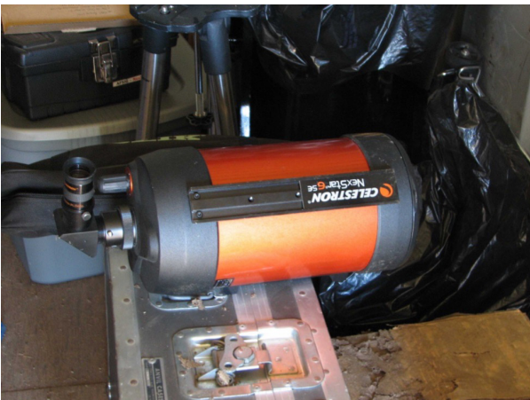
Celestron Nexstar 6" SCT , diagonal, and eyepiece
