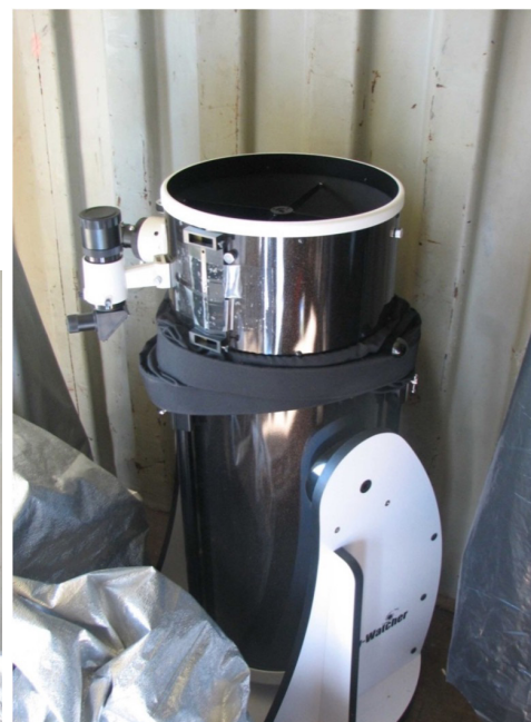
Orion SkyWatcher 12" Collapsible Dobsonian with 8x50 finder
