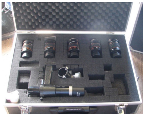
Eyepiece Case #1: Black Orion Case 5 1.25-inch Celestron Multi Coated X-Cell LX eyepieces: 25mm, 18mm, 12mm, 9mm, 7mm focal lengths. 6x30 finder and diagonal.
