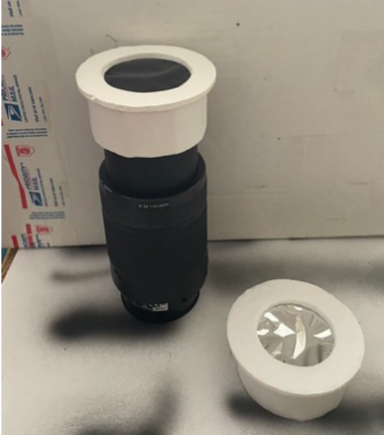
Baader Film on the lower right and Seymour film on a 63mm lens on the left.
