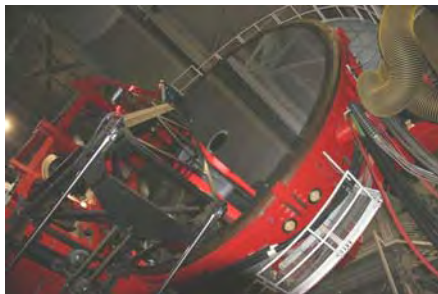
Two views of one of the LBT telescope mirrors. Each image shows one of the 8.4 meter, f/1.14 mirrors.
